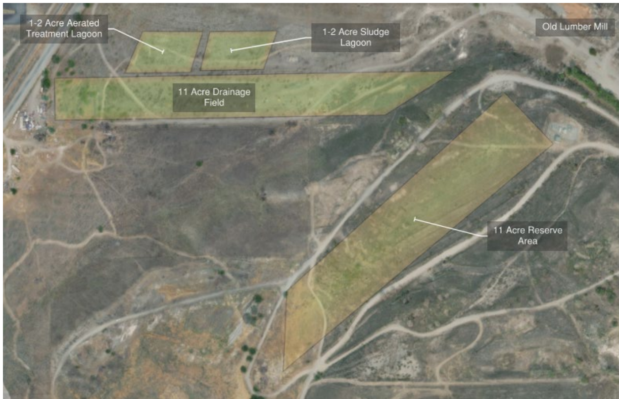
Figure 26. Rendition of Treatment Lagoon & Drainage Fields
