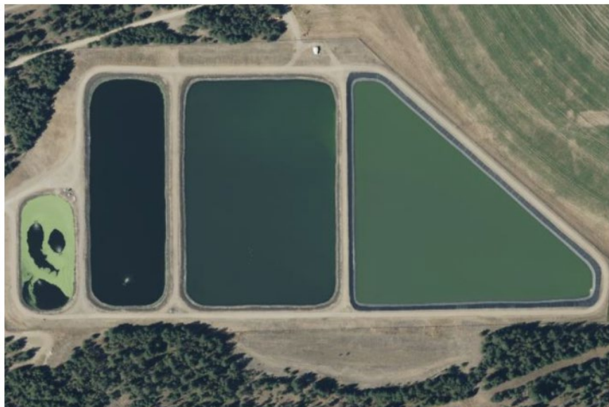
Figure 12. Example of a Lagoon System
