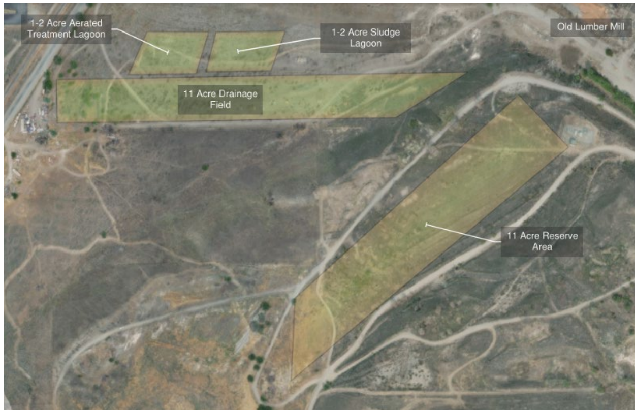
Figure 15. Rendition of Treatment Lagoon & Drainage Fields
