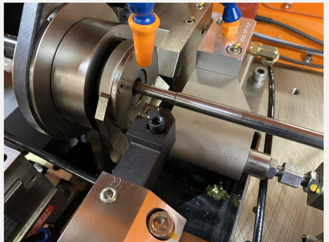
FIG.4 Trim Cutter with air blow off
